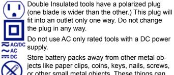
Store battery packs away from other metal objects like paper clips, coins, keys, nails, screws, or other small metal objects. These things can make a connection from one terminal to the other, shorting the battery terminals together and causing burns or fire.
