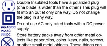
DC supply. Store battery packs away from other metal objects like paper clips, coins, keys, nails, screws, or other small metal objects. These things can make a connection from one terminal to the other, shorting the battery terminals together
