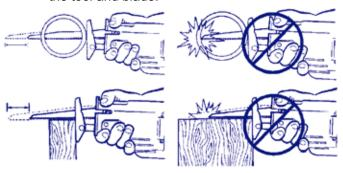
When cutting metal, choose a blade that will allow for at least three blade teeth to be in the material at all times. Less than three teeth will result in teeth snagging and breakage. However, using blades with too fine a tooth will slow your cut.
