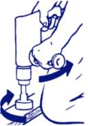
keep the bit cutting or chipping smoothly. If the motor slows down, relieve the pressure. Too much pressure can damage the bit and cause you to lose control of the tool.
